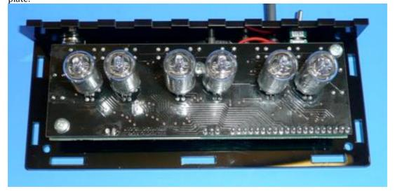
Mount the pcb to the bottom plate using the 3 M3 $\times$ 5 screws with low torque. Test the function of the socket, the switch and the GPS/DCF module.
