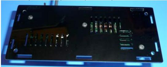
Mount the top plate and fix it from the bottom plate with 4 M3×5 screws.
